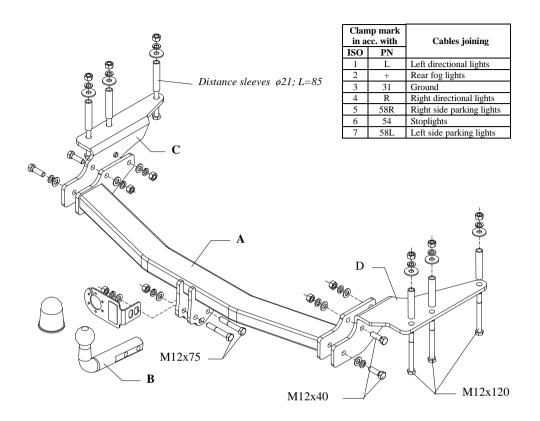
This towbar is designed to assembly in following cars: **SSANG YONG REXTON** produced since 2002, catalogue no. **SY01** and is prepared to tow trailers max total weight **2300 kg** and max vertical load **140 kg**.
